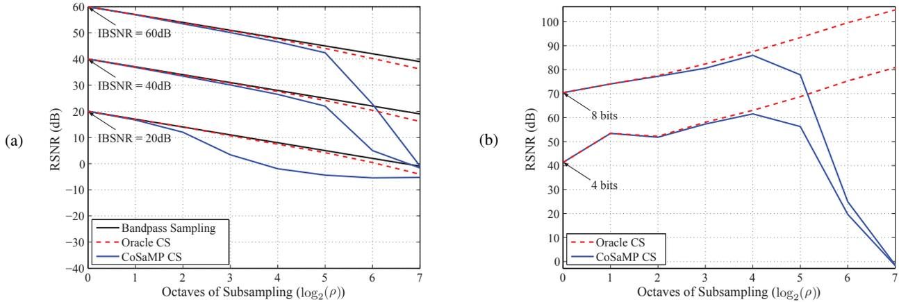
**Fig. 3.** Impact of the noise and quantization on the recovered SNR (RSNR) as a function of the subsampling ratio  $\rho$  and a simple sparse input consisting of a single unmodulated sinusoid. (a) shows the “3 dB/octave” noise figure increase induced by CS, while (b) shows that the DR of the receiver improves with sampling rate reduction by about 6 dB per octave.
