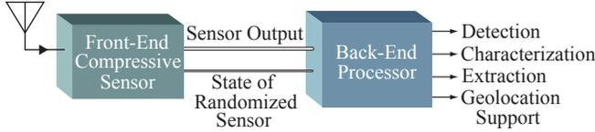
**Fig. 1.** The processing asymmetry assumed in a CS wideband acquisition receiver. The low size, weight, power and cost of the compressive sensor usually implies the need for substantial computation at the “backend” of the system.
