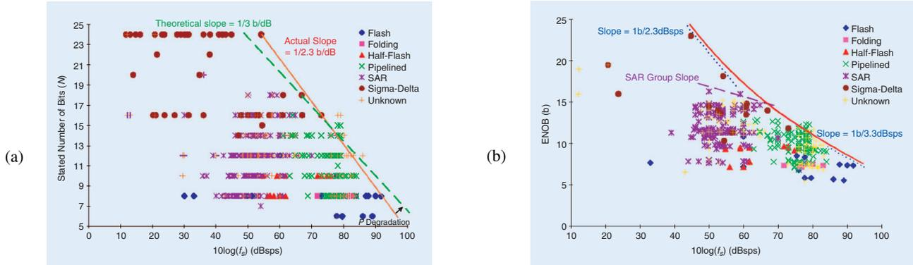
**Fig. 2.** Several studies, including the one illustrated here [11], have shown a clear empirical relationship between the quantization rate achieved by a practical ADC and the precision with it can make its measurements. (a) Stated number of bits vs. sample rate. (b) Effective number of bits (ENOB) vs. sample rate. Figure courtesy of [11].
