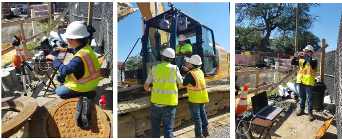
Figure 3: Setup process for audio collections using microphone array (left) and contact microphone (middle); Simultaneous video recording for generating the ground truth data (right).
