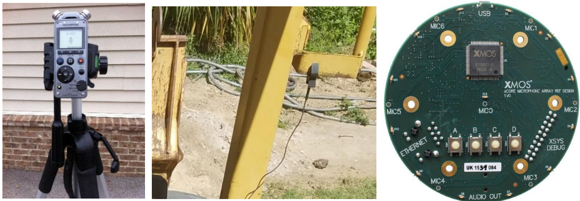
Figure 1: Different types of microphones used in the project: Zoom H1 digital handy recorder mounted on a tripod (left); Korg CM-200 clip-on contact microphone attached to CAT loader (middle); xCORE-200 microphone array evaluation board – top (left).
