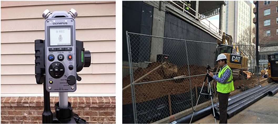
Fig. 4. The microphone array used for collecting audio files for this project (left) and placing audio recorders at a jobsite (right).
