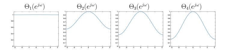
Notice that the spectrum is flat for L = 1 — this is because superimposing the  $b_1(t)$  also does linear interpolation. For the other values of L, the inverse is very well conditioned. We set
