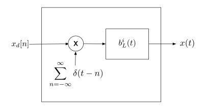
The  $b_L^i(t)$  are called the interpolating splines, or the *cardinal spline* functions. Here is a sketch of the cardinal spline for L = 3:
