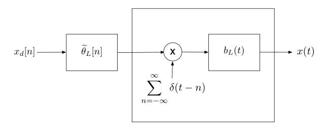
We can combine this into a single block as follows. The impulse response of this system (what comes out when  $x_d[n] = \delta[n]$ ) is
