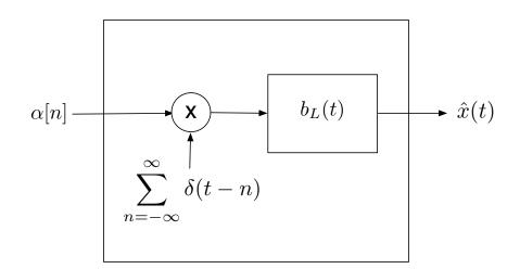
So just as it is possible to reconstruct bandlimited signals from uniform samples, splines with equally spaced knots can also be reconstructed from uniform samples (after pre-filtering).
