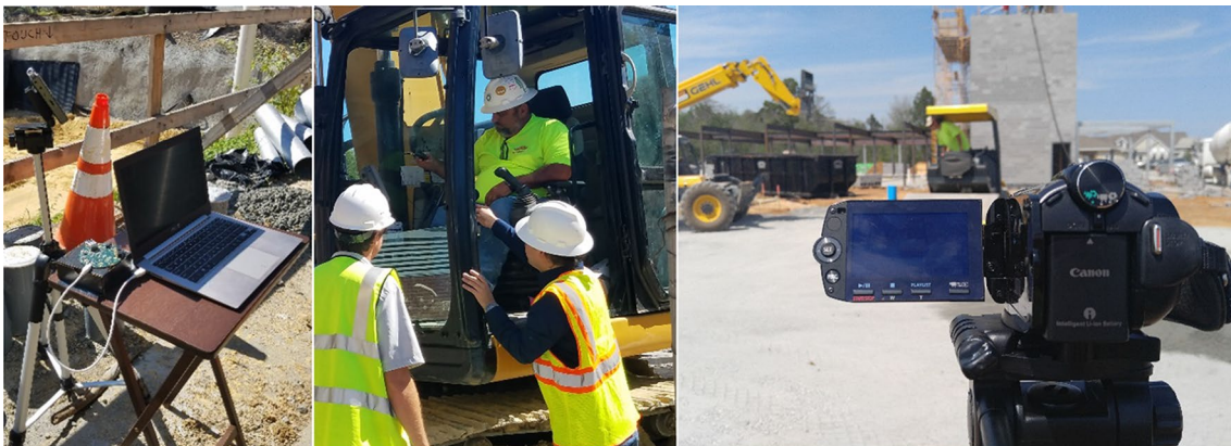
Fig. 8 Setup process for audio collections using microphone array and off-the-shelf microphone on-site (left), and contact microphone and off-the shelf microphone onboard (middle); simultaneous video recording for generating the ground truth data (right)
